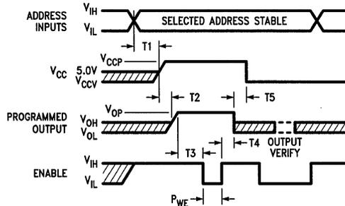
NOTE: ENABLE WAVEFORM FOR AN ACTIVE LOW ENABLE. SOME PROMS HAVE MORE THAN ONE CHIP ENABLE. HOLD ALL OTHER ENABLE(S) TO ACTIVE STATE(S).
