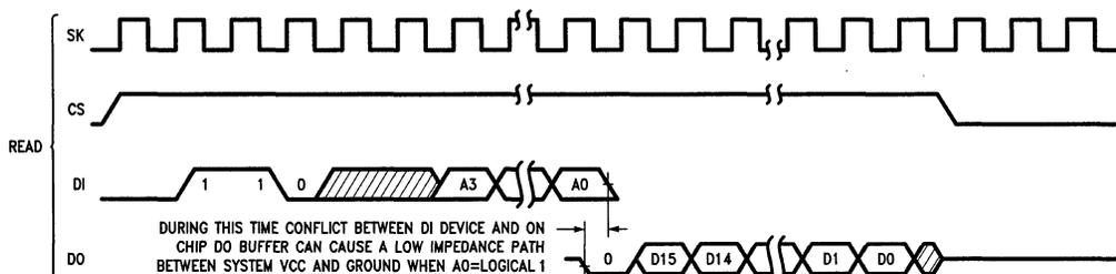
FIGURE 1. Read Instruction in Common I/O Configuration
