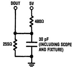
FIGURE 1. Output Load
