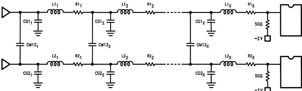
FIGURE 9. RLCM Network Model for PCB (Unloaded)
