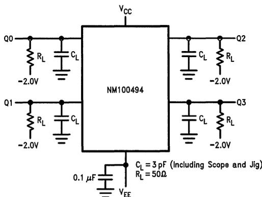
FIGURE 2. AC Test Circuit
