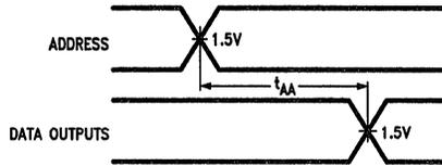
**3b. Read Mode Propagation Delay from Address**
