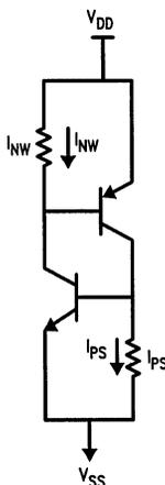
FIGURE 2. Parasitic Bipolar Schematic
