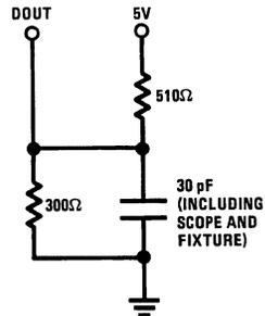
FIGURE 1. Output Load
