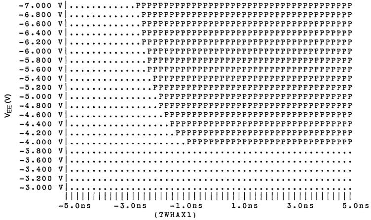
FIGURE 1. Address Hold Time vs Operating Supply Voltage
