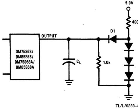
$C_L = 5.0 \text{ pF}$  for  $t_{HZ}$ ,  $t_{LZ}$
