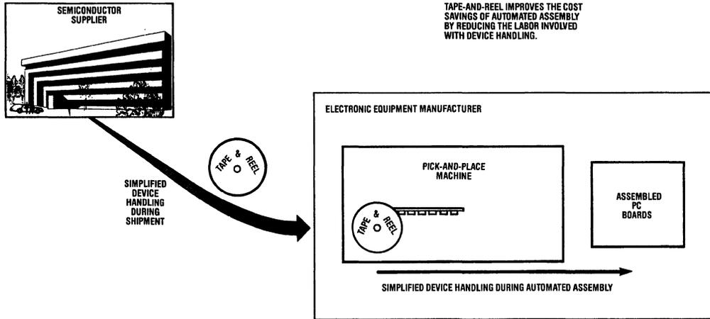
TAPE-AND-REEL IMPROVES THE COST SAVINGS OF AUTOMATED ASSEMBLY BY REDUCING THE LABOR INVOLVED WITH DEVICE HANDLING.
