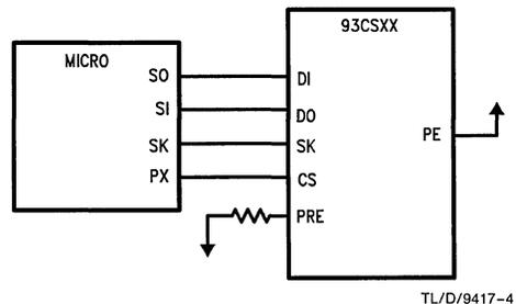
FIGURE 2b. Protect Register Enabled with Pulldown
