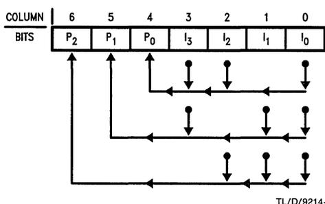
FIGURE 1. Computation Scheme for Parity Bits Using Hamming Code
