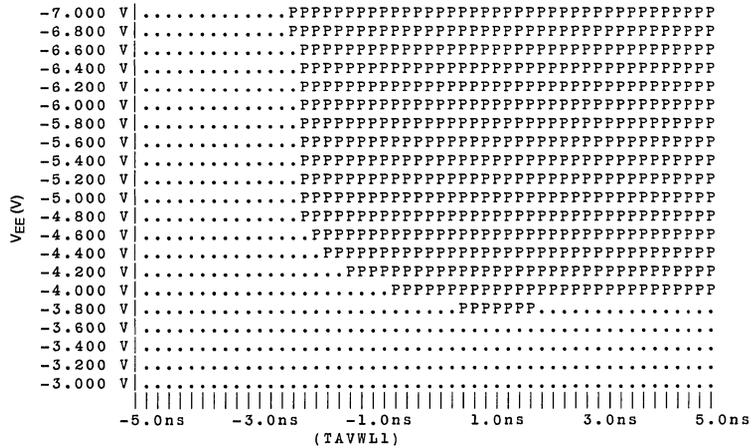
FIGURE 2. Address Setup Time vs Operating Supply Voltage
