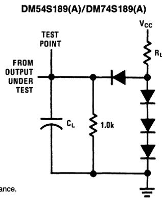
$C_L$  includes probe and jig capacitance.
