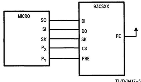
FIGURE 2c. Protect Register Enabled
