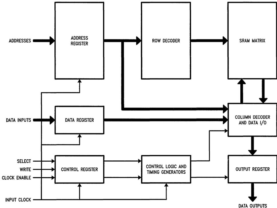
FIGURE 6. Advanced Self-Timed SRAM Simplified Block Diagram
