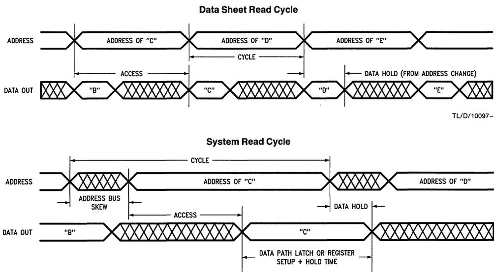
FIGURE 1. Generic SRAM Read Timing
