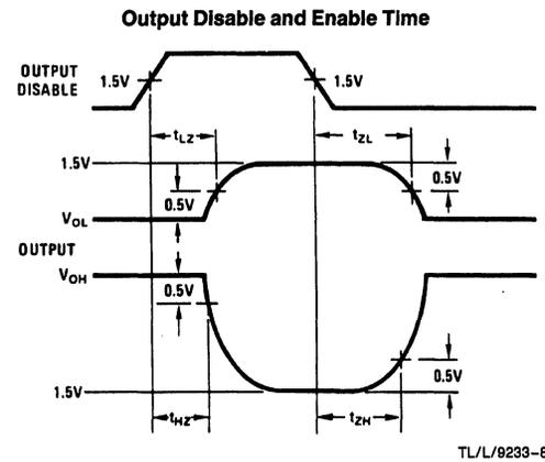
**Note:** Input waveforms supplied by pulse generator having the following characteristics:  $V = 3.0V$ ,  $t_r \leq 2.5 \text{ ns}$ ,  $PRR \leq 1.0 \text{ MHz}$  and  $Z_{OUT} = 50M$ .
