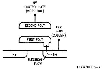
**FIGURE 6. Write Operation**
