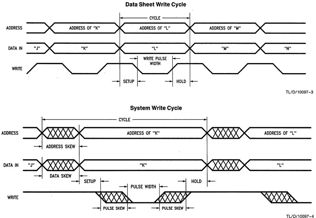
**FIGURE 2. Generic SRAM Write Timing**
